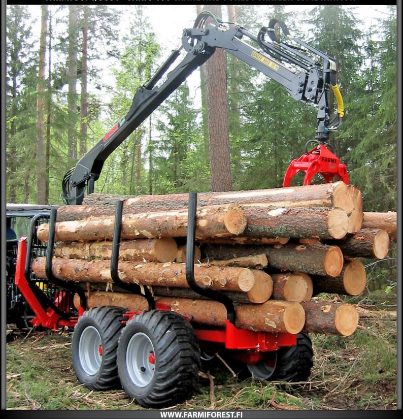
The far-reaching FARMI 5871/5881 log loader mounted on the FARMI 101 forest trailer make a suitable forwarder combination for everyday work on forest terrain of all types. Thanks to their modular structure, accessories can be added according to the customer's needs. The recommended amount of timber transferred is 5,000–12,000 m3/year.
