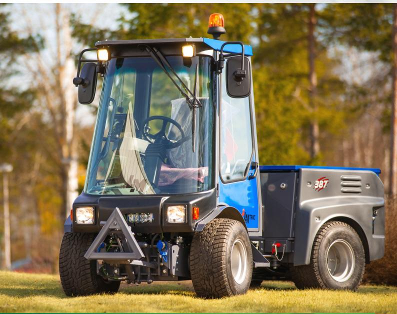
LM Trac 387 is a handy machine in city environment. Small turning circle and narrow construction prove effective on cramped streets and alleys.
